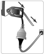
3. Once the cable is fitted, pull firmly on the cable side shown to locate securely.
